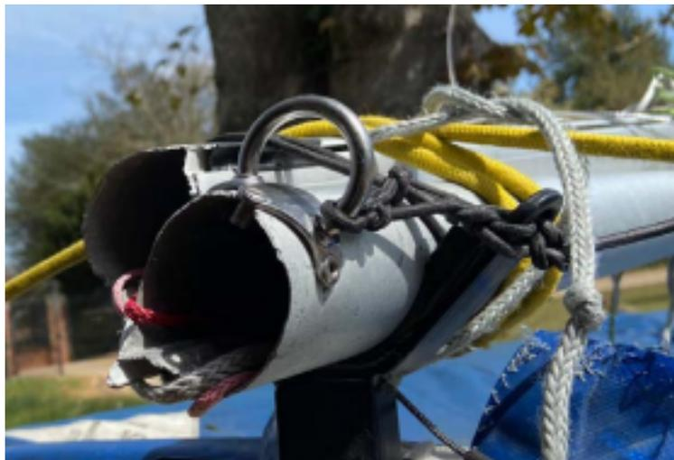
This is an unusual place for a part to go, however the coaches have been having a chat and we think that this failure has probably occurred due to corrosion around the fitting on the mast over time.
